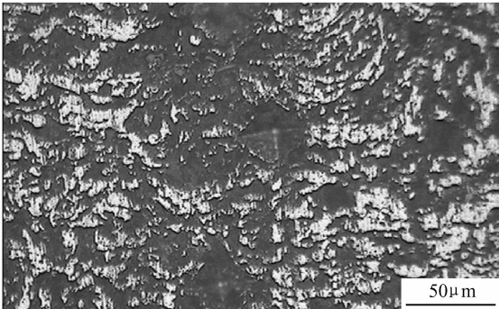
图 5 高速电弧喷涂 Al-RE 涂层的截面形貌(混合酸腐蚀) Fig. 5 Cross-section metallograph of the high velocity arc sprayed Al-RE coating (etched with mixed acid)
