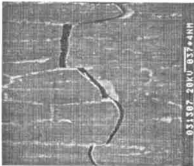
图 4 纤维独石陶瓷材料裂纹偏转的显微照片 Fig. 4 SEM micrograph of crack deflection in fibrous monolithic ceramic
