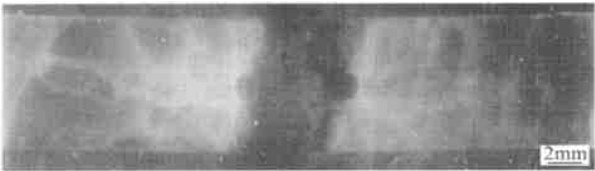
图 1 孔径 5mm 层合板疲劳失效试件的 X 射线图 Fig. 1 X-ray graph for a tensile specimen with a hole in diameter 5mm
