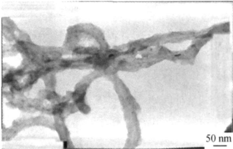
图 4 水介质环境中原位化学氧化合成 PEDOT 包覆 CNTs 的 TEM Fig. 4 TEM image of CNTs capsulated by PEDOT in-situ polymerization in water
