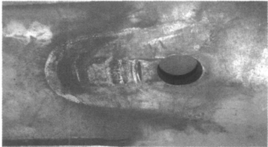
图 8 拖把头下耳片被舌状耳片挤压痕迹 Fig. 8 Contact marks on towbar lower attachment
