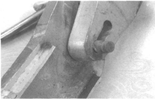
图 7 拖把插销被舌状耳片耳孔边缘挤伤 Fig. 7 Contact marks on pin by middle attachment
