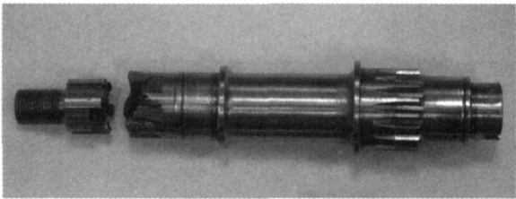
图 1 断裂花键轴外观形貌 Fig. 1 Macrograph and fracture position of spline shaft
