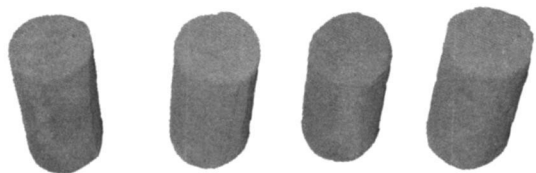
图 2 CIP 后的圆柱体试样 Fig. 2 Column after CIP
