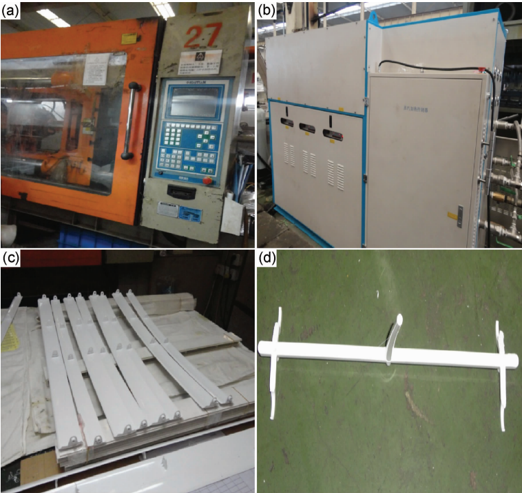
图 6 导风板实验生产 (a)注塑机;(b)蒸汽加热控制器;(c)导风板;(d)浇注系统凝料 Fig. 6 Wind deflector production (a)injection molding machine; (b)steam heating controller;(c)wind deflector;(d)runner system
