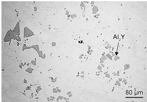
图 2 AZ91-Y 试样中 \text{Al}_2\text{Y} 颗粒相 Fig. 2 \text{Al}_2\text{Y} particles phase of AZ91-Y sample
