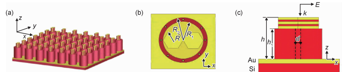
图 5 用于太阳能的吸波器结构示意图 [43] (a)周期性结构单元;(b)俯视图;(c)侧视图 Fig. 5 Schematic diagrams of the structure of the absorber for solar energy [43] (a)periodic structural element;(b)top view;(c)side view
